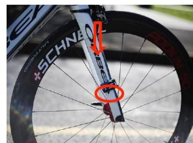
Mount as low as practicable on either fork
